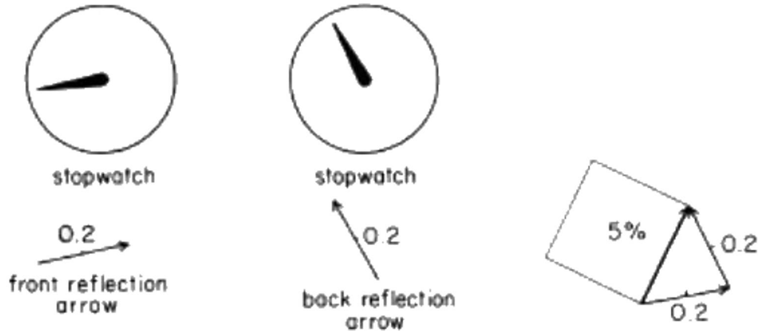
FIGURE 13. The final arrow for a slightly thicker sheet of glass is a little longer, due to the greater relative angle between the front and back reflection arrows. This is because a photon bouncing off the back surface takes a little longer to reach A compared to the previous example.
