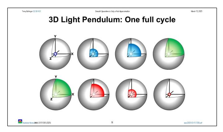
[25:51] Here's a 3D light pendulum. I like this thing! You have a light emitter at the center of [a reflective] sphere. [It emits] a pulse of light that goes out in all directions, bounces [off the inner surface of the sphere and] returns [to a detector co-located with the emitter at the center.]
